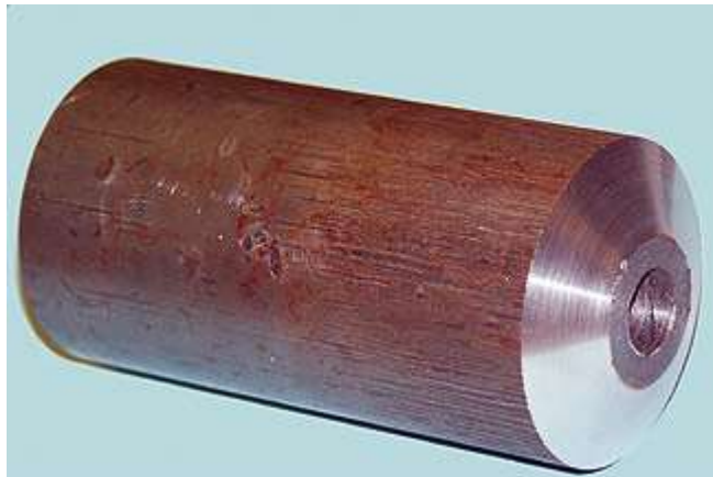
Fig. 1: The skate above is made from a newsprint roll shaft.
