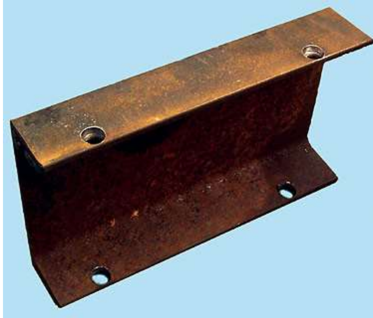
Fig. 2: Holes drilled closer to the ground will improve the skate's safety.
