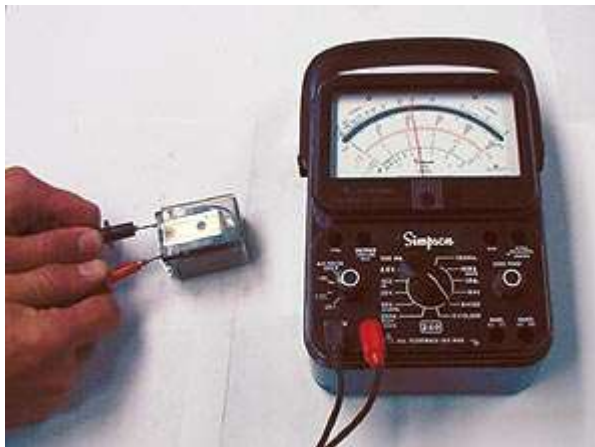
Fig. 4: How to test a coil.
