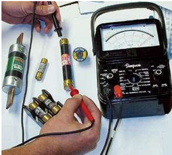
Fig. 3: Working fuses yield a resistance of less than 1 ohm.
