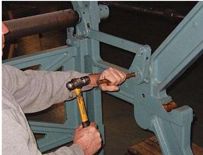
Fig. 5: Removing the shaft.
